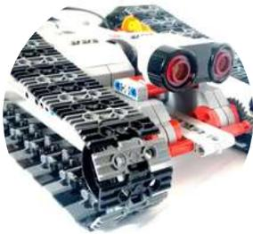
Campers will learn about design requirements to build vehicles that are able to scale steep inclines (think dune buggies in hill climbing, hill climbing motorcycles, etc.) and then will design, build, test, and compete with their hill climbing robot on a steep incline. Students will also 3D design/3D print components including wheelie bars to better keep their Hill Climbing robot from flipping over!
